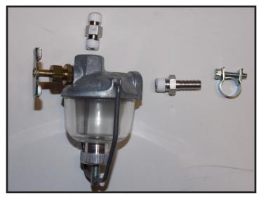
type, and why one type is better for our motorcars than others. We want a style that has a shut-off valve with a back-stop and a large handle/knob. When it is open all the way it stops turning, showing it can't turn any further out and won't vibrate out and get lost. You don't need to strong-man the valve closed or open, two finger should be enough.
