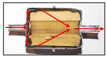
season weather you think it is bad or not. Reliability is more important than a \$10 (or less) fuel filter. I always carry 2 new units with me, one for me and one for a fellow motorcar operator in need. The paper inside these filters is called 'hydroscopic', meaning it will absorb water until the filter paper becomes swollen and the fuel will all but stop flowing. Those plastic shell fuel filters can't take any heat and get brittle fast and can
